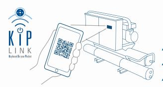
As an option, the direct control over the unit comes through the innovative KIPlink interface. Based on Wi-Fi technology, KIPlink gets rid of the standard keyboard and allows one to operate on the unit directly from a mobile device (smartphone, tablet, notebook).
